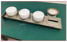
Fig. 6 Four-element antenna array with rounded rectangular slots.
