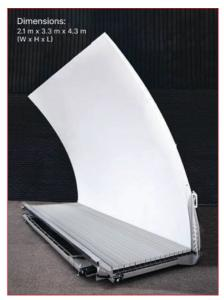
Fig. 1 The RanLOS test system for vehicular applications.
