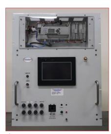
▲ Fig. 1 Front panel of TR-3600 Solid-State Weather Radar Transmitter.
