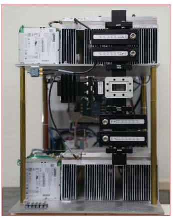
OCAI Fig. 2 Back view of TR-3600 Solid-State Weather Radar and Transmitter.
